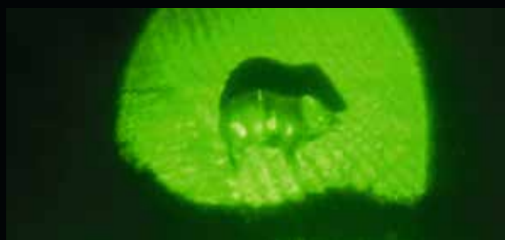
When the terrain is unfavourable, an illuminated circle can reflect the ground: an undesirable effect.
