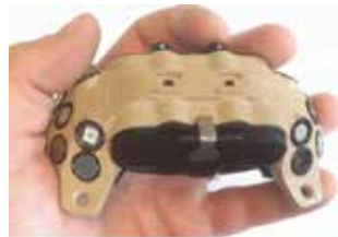
The palm-sized MCID has a low-profile lightweight design that matches the curve of the helmet.
